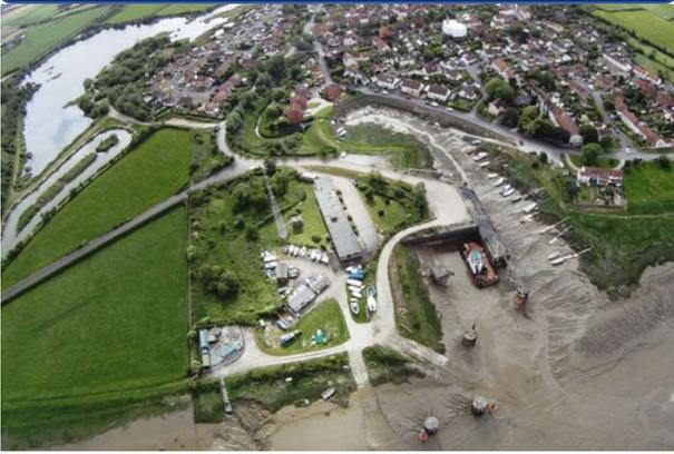
The Combwich Wharf infrastructure in the South West of England was subject to significant refurbishment and modernization. The project created a new berth hardstanding that allows vessels to be unloaded when the tide is out.
